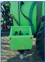
Optional induction hopper with can wash and rinse ring
